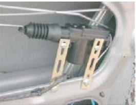
just make sure that the window does not hit the new Door Lock Motor. You will need to drill 2 small holes in the metal inner panel and bend the connecting rod to suit. DO NOT fully tighten the adapter that fixes the new rod to the original connector rod, this will need adjusting once it's all working.
